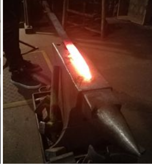
Figure A.10. Hammering Sword on Anvil.
