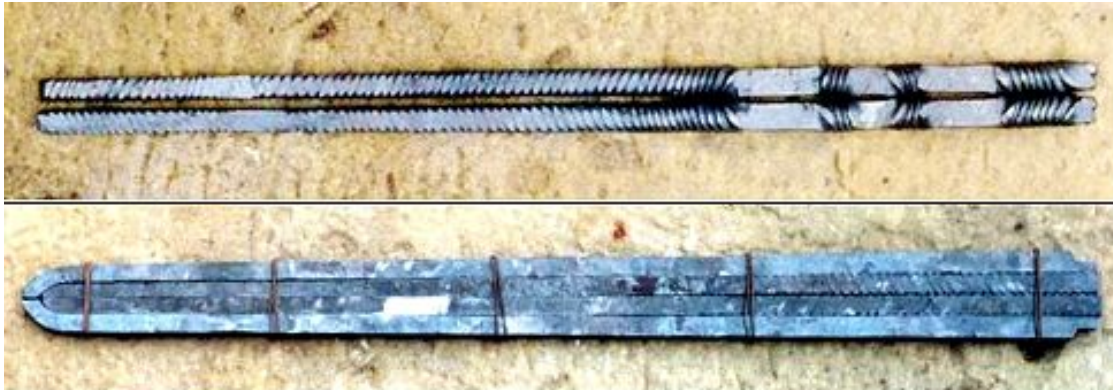
Figure 3.5. Arrangement of Rods For Welding [98].
