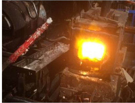
Figure 5.11. Adding Flux to the Hot Metal.
