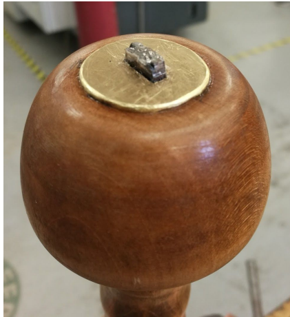
Figure A.27a. Tang Before Peening.
