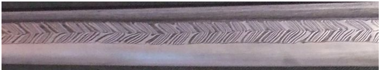
Figure 3.7. Herringbone Pattern Result from Twists Running in Alternate Directions [98].
