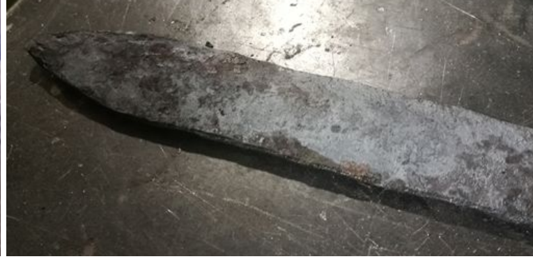
Figure A.12. Sword After Hammering Edges
