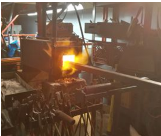
Figure A.7. Propane Furnace.
