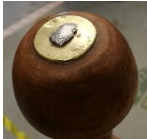
Figure A.27b. Tang After Peening
