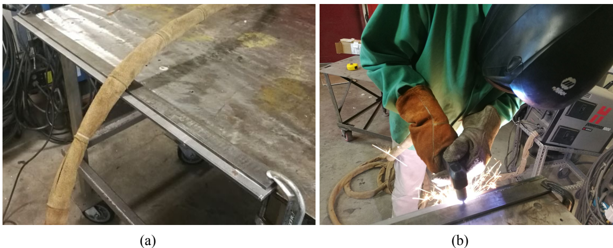
Figure A.3. (a) Original Plate of 1075 Steel and (b) Plasma Cutting the 1075 to the Proper Width.
