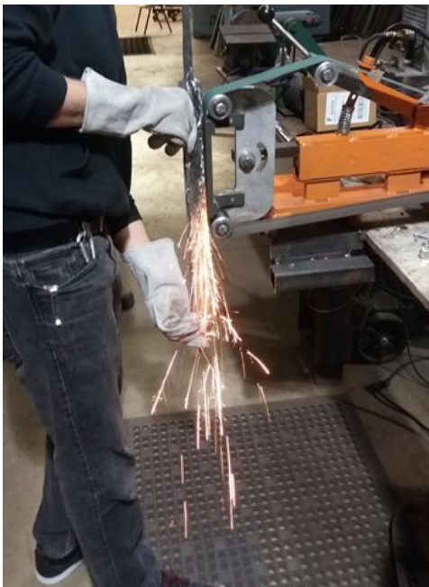
Figure 5.20. Straightening Blade Edge.
