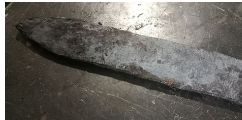
Figure 5.15. Sword After Hammering Edges.
