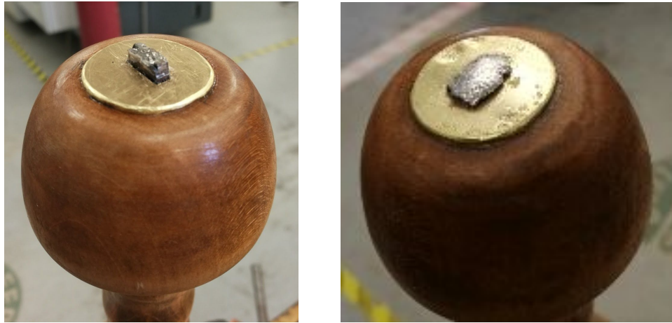
Figure 5.34(a) Tang Before Peening and (b) Tang After Peening.
