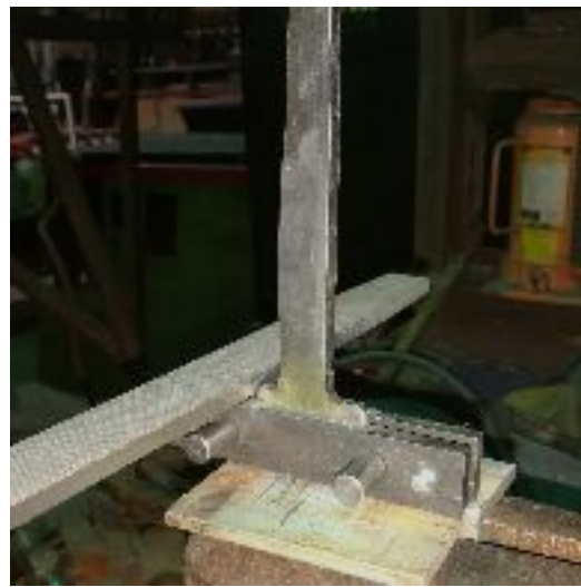
Figure 5.23. Filing Tang Using File Guide.
