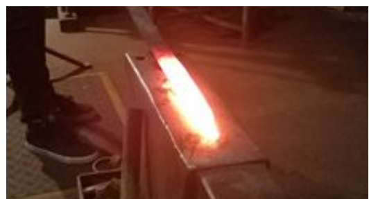
Figure 5.13. Hammering Sword on Anvil.
