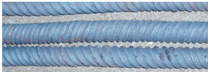
Figure 3.4. Twisted Rods for Modern Pattern Welding [99].
