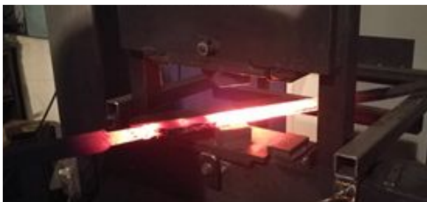
Figure 5.12. Stretching Metal on Pneumatic Press.
