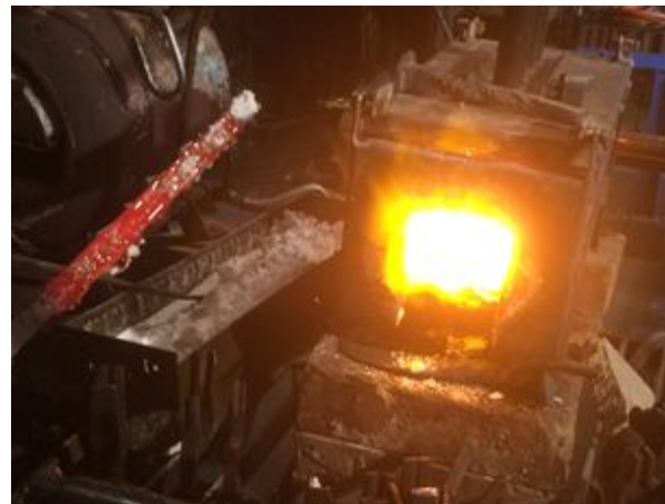
Figure A.8. Adding Flux to the Hot Metal.
