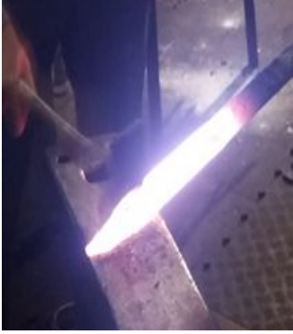
Figure A.11. Hammering the Point.
